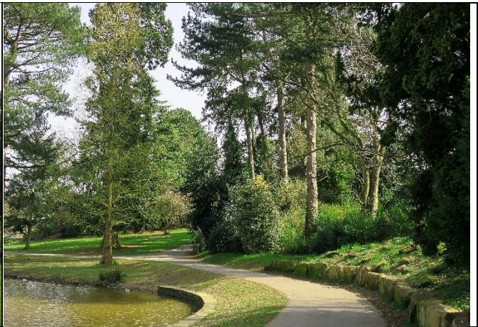
17) 'Rustic' rockwork retains the slope behind and provides permanent edging to the path – a device Kemp used in Congleton Park. Stonework at the lake edge is modern.
